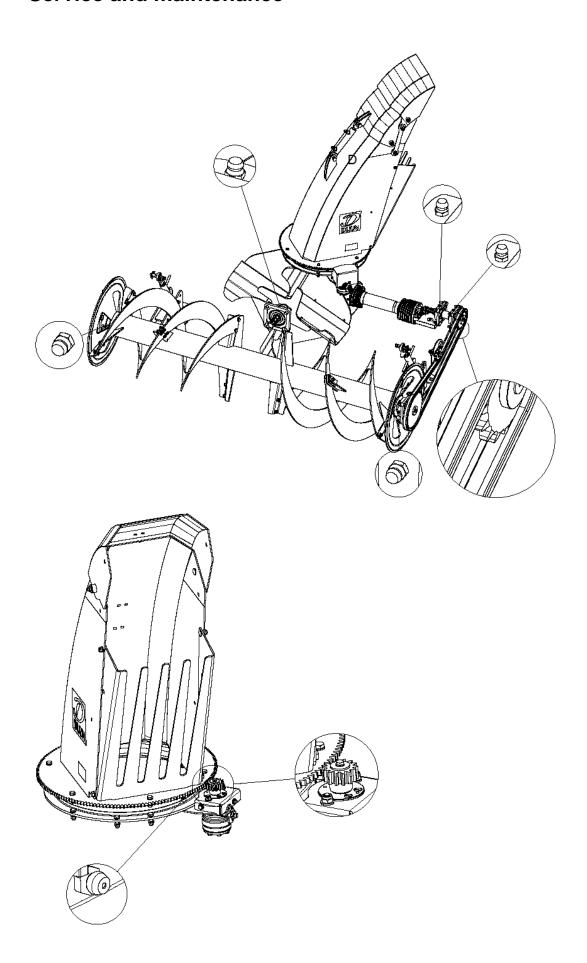
Before cleaning, lubricating, repairing or adjusting the machine, stop the engine and activate the handbrake, and remove the key during work. Close the safety crane on the snow blower that closes the oil on the operation of the feeder screw.
