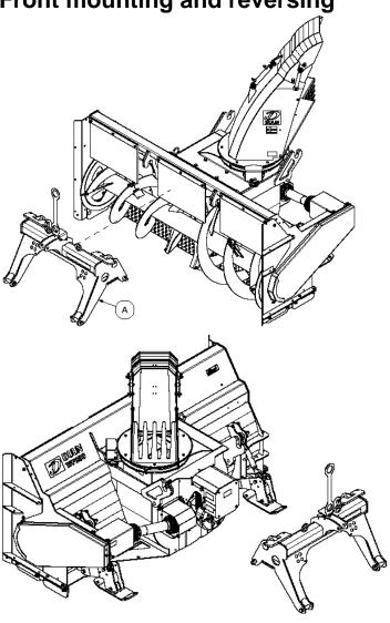
To use snow blower for front mounting or when reversing, the snow blower must change the direction of travel. Changing the direction of travel is done by turning three point linkage to the opposite side of the snow blower. Loosen up two screws that hold the three point linkage and use the tractor to turn it around on the opposite side. Remember to put screws back and secure them.
