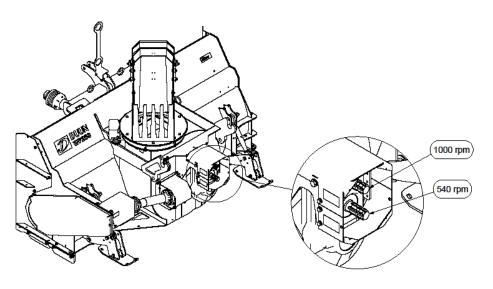
The snow blower is prepared for reversing and front mounting.
